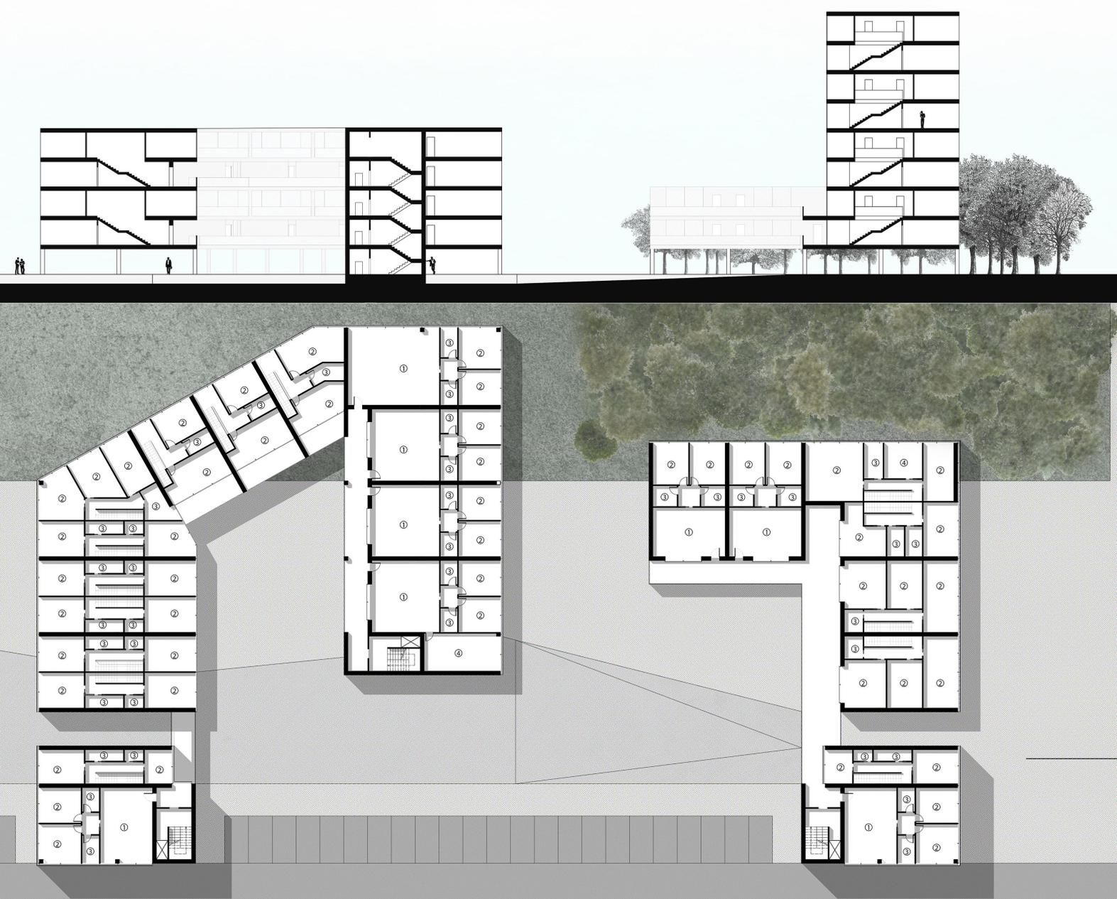
The drawings show a multi-story building with a central core and multiple wings. The floor plans are numbered, likely corresponding to the modular units described in the previous section. The cross-sections illustrate the vertical arrangement of spaces, including a staircase and various levels of the building.
