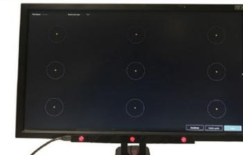
Figure 6.29 An example of a passive eye-tracking device that does not require the user to wear anything. (Photograph courtesy of Joseph J. LaViola Jr.)
